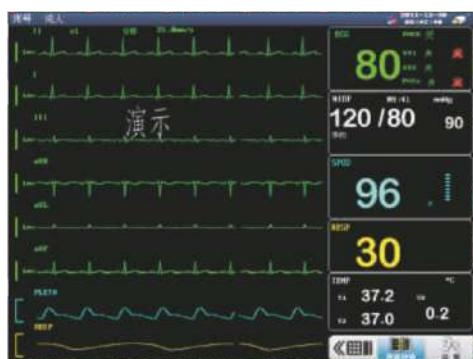
Max 8 waveform display simultaneously,
